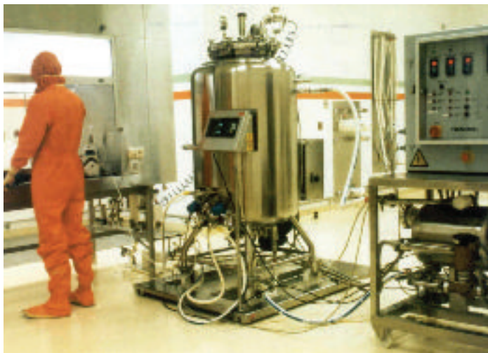
Figure 2: Modern large-scale vaccine production using advanced cell culture techniques (Courtesy of GSK Biologicals)
